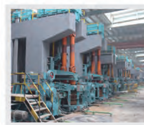
Wire Rod And Bar Rolling Mill
